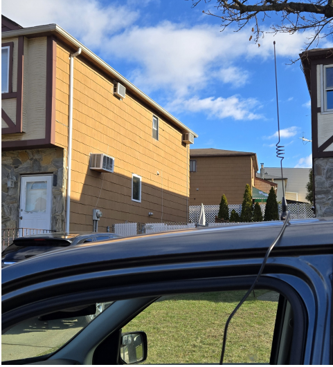
Figure 5: The magnetic mount cellular antenna on the front part of the roof of the vehicle is connected to the tinySA. The GPS tracker is magnetically attached underneath the front bumper of the vehicle.
